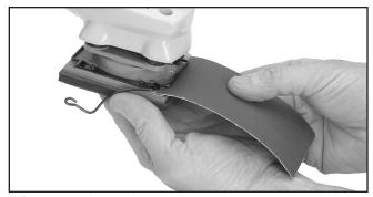
Figure 3. Attaching and securing sanding sheet.
